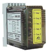
The temperature settings can be adjusted on the relay in the electrical cabinet. On the relay are 5 potentiometers. To adjust the temperature, the switch must be in the coressponding position. Turning clockwise will set the temperature up, turning counter-clockwise will set the temperature down. The pre-set temperature will be shown at the controller. The information sign should be indicated according to the set temperatures.
