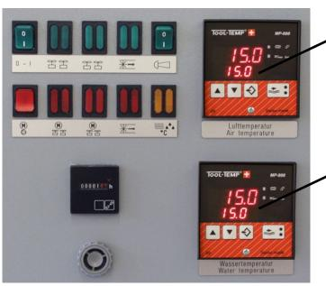
**Temperature controller for air temperature** As soon as the set temperature is exceeded, the complete unit switches off.
