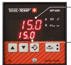
Set temperature / required temperature Adjustable in  $^{1}/_{10}^{\circ}$  range
